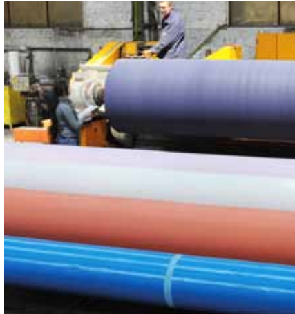
RiWaMat composite ceramic cover on the grinding machine
