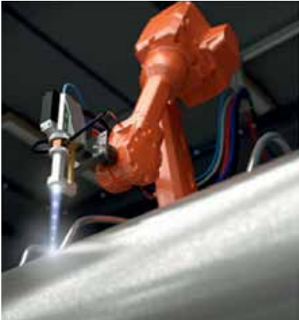
RiWaMat calender roll Tungsten carbide coating by HVOF process
