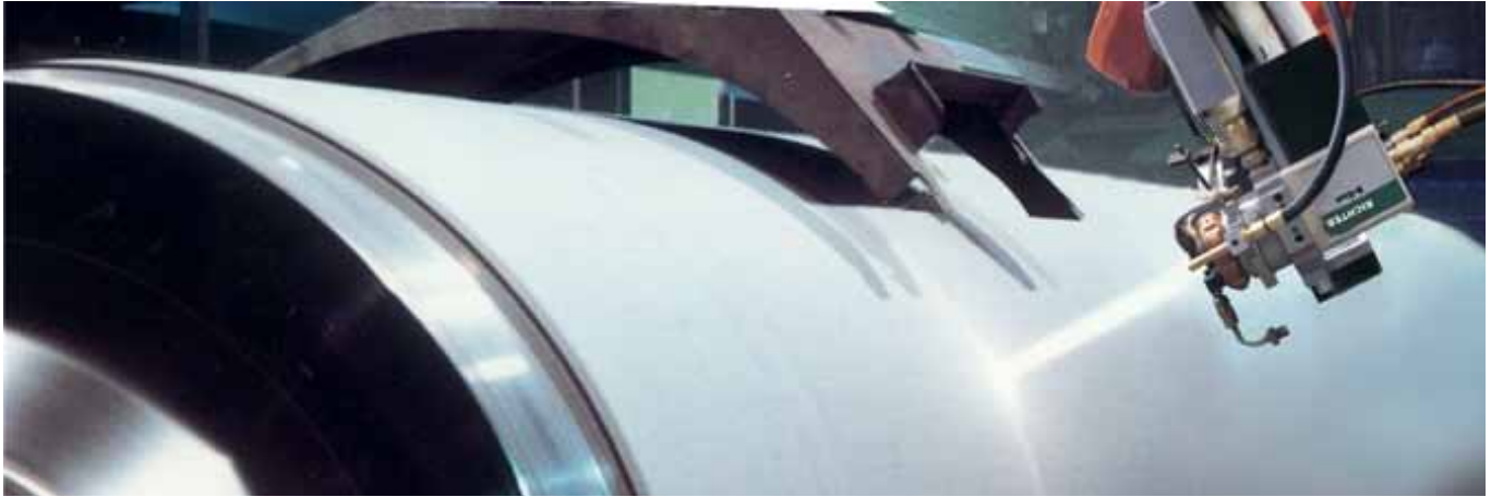
RiWaMat center roll ceramic coating by Plasma process
