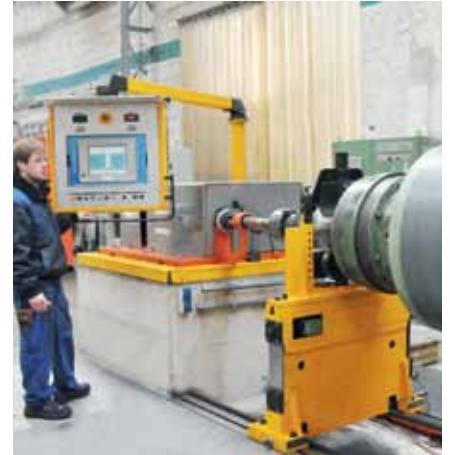
Plasma ceramics center roll on the dynamic balance machine
