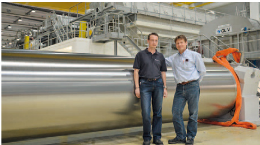
View of the G-cover of UPM Hürth coated with hard metal
