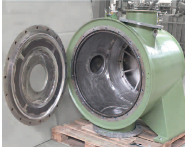
Highly wear-resistant regenerated F1TFiberizer housing processed on a CNC mill machine
