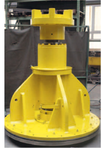
Pulper storage Escher Wyss ST11 after general overhaul
