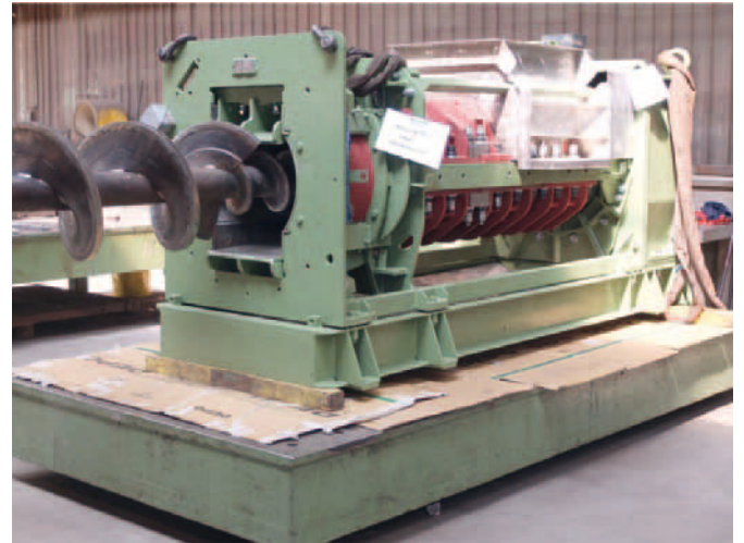
General overhaul of a BP601 Beltec press highly wear-resistant press BP601 [sic.: with components reworked to be highly wear-resistant]
