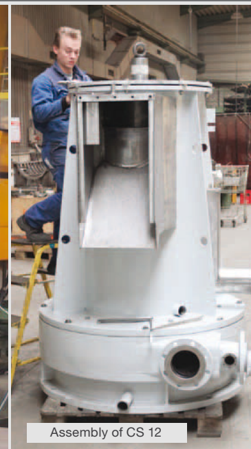
Processing of a new „wear resistant“ top part of the housing Combisorter CS12
