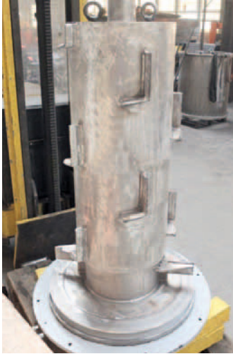
Drum rotor CS12 (see title page), reworked to be highly wear-resistant
